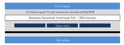
• Front-glass can be replaced by an ETFE frontsheet material with adequate adhesion properties.
